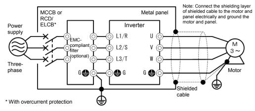
Figure H.1- 1 Mounting an EMC-compliant Filter (option) in a Metal Panel
