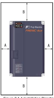
Figure 2.1-1 Installation Direction
