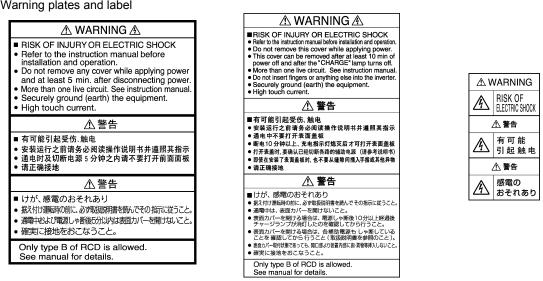
(a) FRN0072E2S-4□ (b) FRN0203E2S-4□ Figure 1.2-2 Warning Plates and Label
