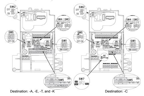
Figure 2.2-20 Various Switch Positions on the Control Printed Circuit Board
