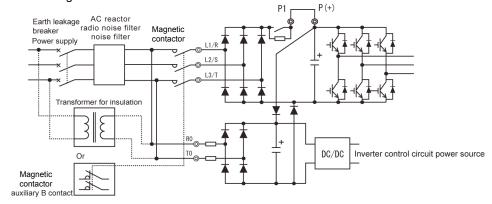
Figure 2.2-5 Connection of the Earth Leakage Breaker
