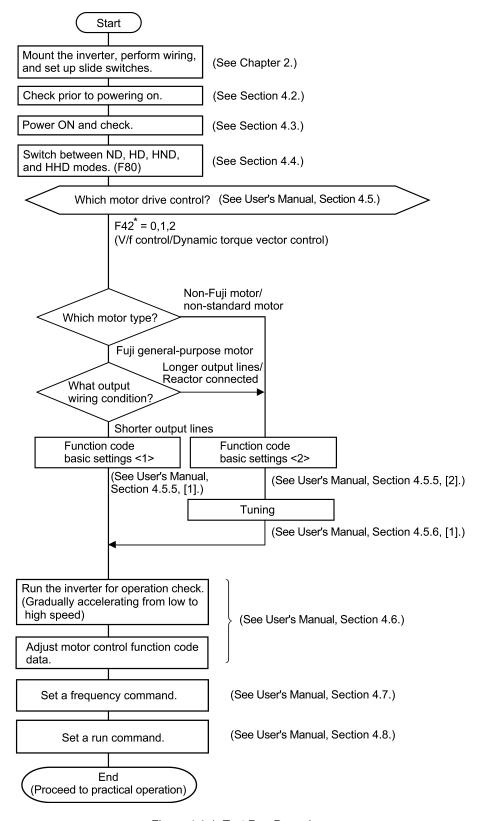
Figure 4.1-1 Test Run Procedure
