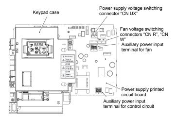
Figure 2.2-18 Switching Connector Positions
