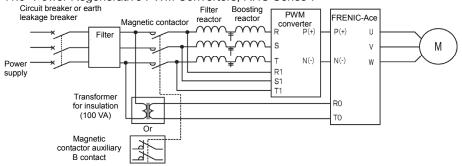
Figure 2.2-6 Example of Grounding in Combination with PWM Converter
