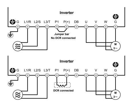
Figure 4.2-1 Connection of Main Circuit Terminals
