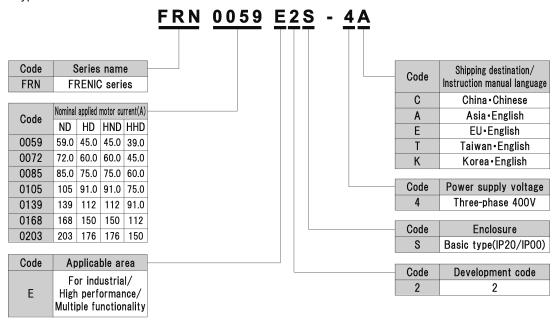
In this manual, inverter types are denoted as "FRN\_ \_ \_ \_ E2S-4 ..." Note
